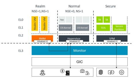
NS = Non-Secure – NSE = Non-Secure Extension RMM = Realm Management Monitor TA = Trusted App – TOS = Trusted OS SPM = Secure Partition Manager GIC = Generic Interrupt Controller
